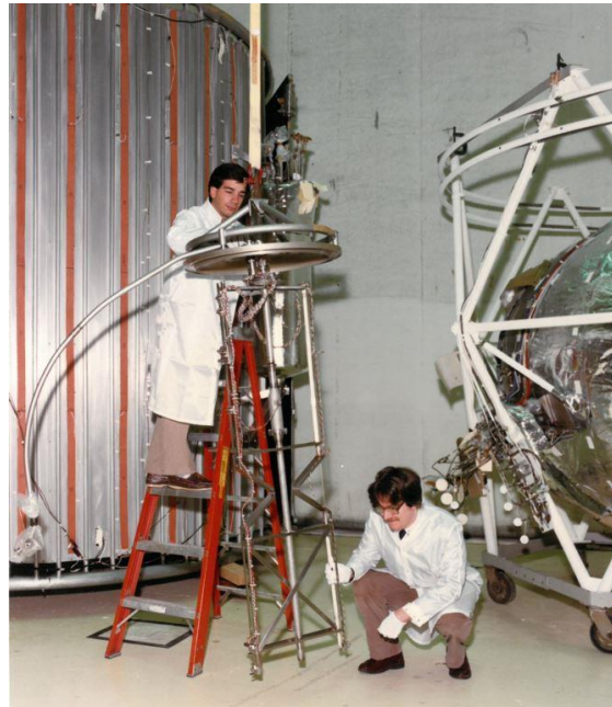
Figure 1. Engineers preparing an array of temperature sensors, or temperature sensor rake for installation at NASA's Glenn Research Center's Armstrong Test Facility.
